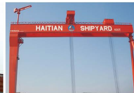
舟山海天船业 400T 造船门机 Zhoushan Hatian Ship Industry 400T Shipbuilding Door Type Crane
