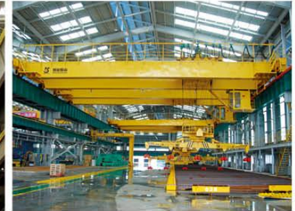
QL 型电磁挂梁桥式起重机 (下旋转) QL Type Electromagnetism Bridge Crane(unrotate)
