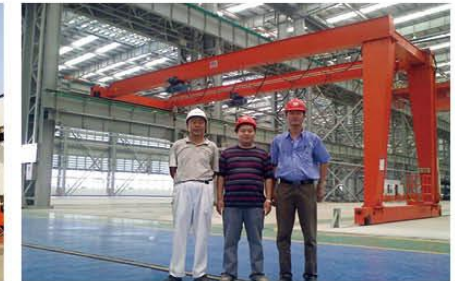
青岛武船重工 10+10T 双梁双葫芦半龙门 Qingdao Wuchuan Heavy Industry 10+10T Double Beam Double Hoist Half Door Crane
