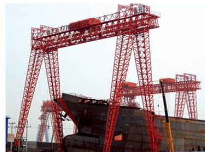
台州枫叶船业 150T 造船门机 Taizhou Fengye Ship Industry 150T Shipbuilding Door Type Crane
