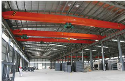
LD 型电动单梁桥式起重机 LD Type Single Girder Electric Bridge Crane
